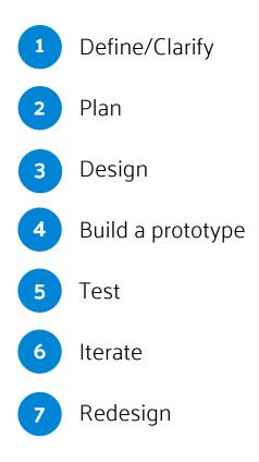
It is a process that can be applied to any problem. Rapid prototyping fits into step 4 - *"Build a prototype"*.
